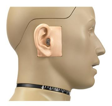
Connection: Traditional Power Supply (200 V/LEMO) Channel(s): 2 ANSI: S3.36 ITU-T Rec. P.57 Type 3.3 based on ITU-T Rec. P.58 The 45BB-3 KEMAR Head and Torso for Sound Quality Recording is an acoustic research tool with built-in 1/2" microphones for realistic sound quality testing and recordings. It is easy ro replace the 1/2" microphones with 1/4" microphones if preferred. Its CCP equivalent is <u>GRAS 45BB-4 KEMAR Head & Torso for Sound Quality</u> <u>Recording, 2-Ch CCP.</u>
