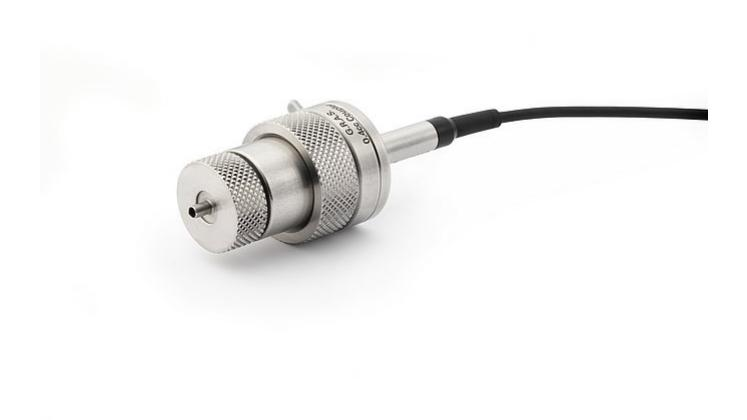
Connection: LEMO Volume: 0.4cc IEC: 60318-8 Use: For hearing aid test up to 16 kHz The GRAS 43BA-1 is a 1/4" 0.4cc High frequency coupler for test of hearing aids. It uses a 1/4" microphone and a 1/4" preamplifier with LEMO connection. The 43BA-2 is the equivalent CCP version.
