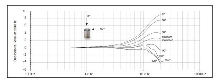
Free-field corrections for different angles of incidence
