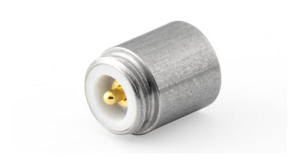
Length: 8 mm Inner threading for preamp.: 5.70-60 UNS-2 Outer threading for mic.: 5.70-60 UNS-2 Material: stainless steel Straight adapter, length 7.5 mm, for placing between a 1/4" microphone and a 1/4" preamplifier. This item is an extender (not adapting anything).
