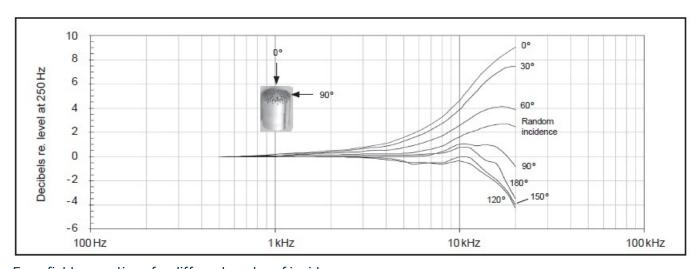
Free-field corrections for different angles of incidence
