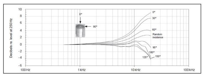
Free-field corrections for different angles of incidence
