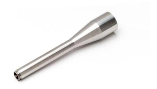
Length: 70 mm Inner threading for preamp.: 11.70-60 UNS-2 Outer threading for mic.: 5.70-60 UNS-2 Material: stainless steel The RA0019 is an adapter for using a 1/4" microphone with a 1/2" preamplifier. Its influence on the acoustic field is minimal. To reduce attenuation of the microphone signal, the guard ring of the preamplifier is extended through the RA0019.
