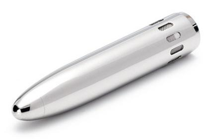
Length: 36.7 mm Outer diameter: 7.35 mm Threading (mic. protection grid threading): M 6,5x0,2 Material: stainless steel Weight: 7 g The RA0026 is specially designed and optimized for use with 1/4" microphones for sound pressure measurements, when high speed wind comes from one known direction e.g. in a wind tunnel.
