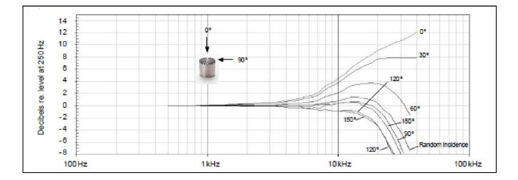
Free-field corrections for various degrees of incidence
