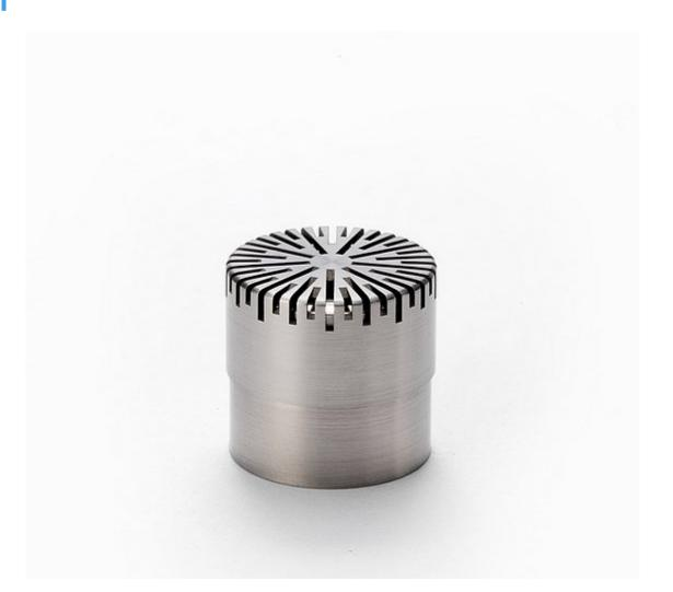
Freq range: 3.15 Hz to 40 kHz Dyn range: 20 dBA to 164 dB Sensitivity: 12.5 mV/Pa The 40AC is an IEC 61094 WS2F classified ½" externally polarized free-field, wide-frequency microphone with rear-venting. The prepolarized equivalent is GRAS 40AM.
