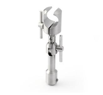
Material: Stainless steel Dimension: For 1/2" Special feature: Adjustable in 45 degree steps The GRAS RA0093 is an adapter for mounting a microphone set (microphone/preamplifier) on tripods having a standard 1/4" UNC-20 male thread. The adapter is provided with a clamp for attaching a 1/2" diameter preamplifier. The microphone can be set in angles between 0 and 180 degrees in 45 degree steps.
