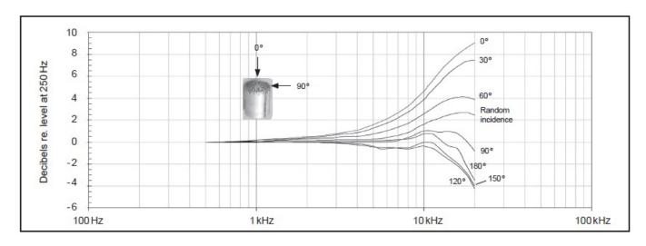
Free-field corrections for different angles of incidence
