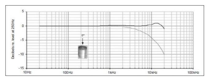
Typical frequency response. Upper curve shows free-field response for  $0^{\circ}$ , lower curve shows pressure response.
