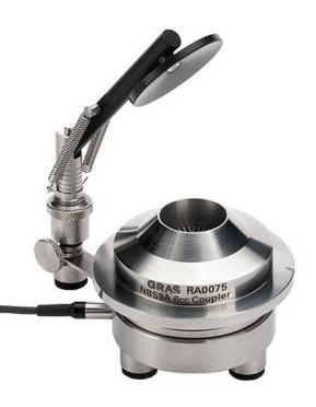
Connection: 200 V/LEMO Volume: 6 cc Dyn range: 14 dB(A) to 146 dB ANSI: S3.7 IEC: 60318-3 The GRAS 43AF-S1 Artificial Ear is a complete test jig for acoustically testing telephone handsets and earphones and complies with ANSI S 3.7 – 1995 – American National Standard for Testing Earphones.:
