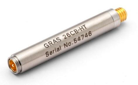
Freq range: 2.5 Hz - 200 kHz Noise: 1.8 µV Gain: -0.35 dB Special feature: High temperatures The GRAS 1/4 preamplifier is a general-purpose preamplifier optimized for use with prepolarized condenser microphones. It is a small, robust unit and uses a GRAS CCP power supply, e.g., GRAS 12AL. It has a very low inherent noise level, a large dynamic range, and a frequency response from below 2 Hz to above 200 kHz.
