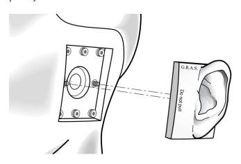
GRAS anthropometric pinna mounted on the 43AG test fixture's cheek plate using the RA0517 kit and finger screws (both included with the anthropometric pinna):
