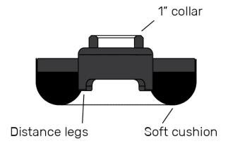
The adapter fits sound calibrators and pistonphones fitted with 1" collar.
