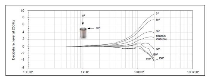
Free-field corrections for different angles of incidence
