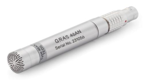
Freq range (±3 dB): 0.5 Hz to 20 kHz Dyn range: 17 dB(A) to 149 dB Sensitivity: 50 mV/Pa Use: For low frequency acoustic diagnostics The GRAS 46AN is a 1/2" Traditional Power (LEMO) freefield microphone set for measuring medium sound pressure levels at low frequencies. It is terminated with a 7-pin LEMO connector and is TEDS compatible. The equivalent Constant Current Power (CCP) type is <u>GRAS</u> <u>46AZ</u>.
