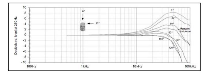
Free-field corrections for different angles of incidence
