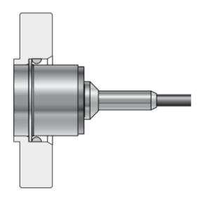
711-style (IEC 60318-4) ear simulator mounted with RA0517 kit on a GRAS 45BB/45BC KEMAR Head and Torso Simulator:
