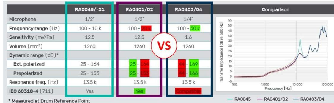
Figure 1. Comparison between RA0401/2 High Frequency ear simulators VS RA0403/4 Hi-Res ear simulators. Green indicates an advantage against the other ear simulator, while red indicates disadvantage.
