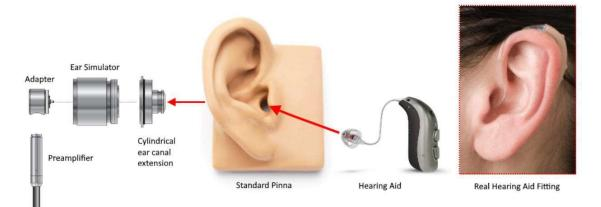
Figure 1. Standard pianne were designed to test hearing aids or in-ear communication devices with conical or cylindrical fittings.
