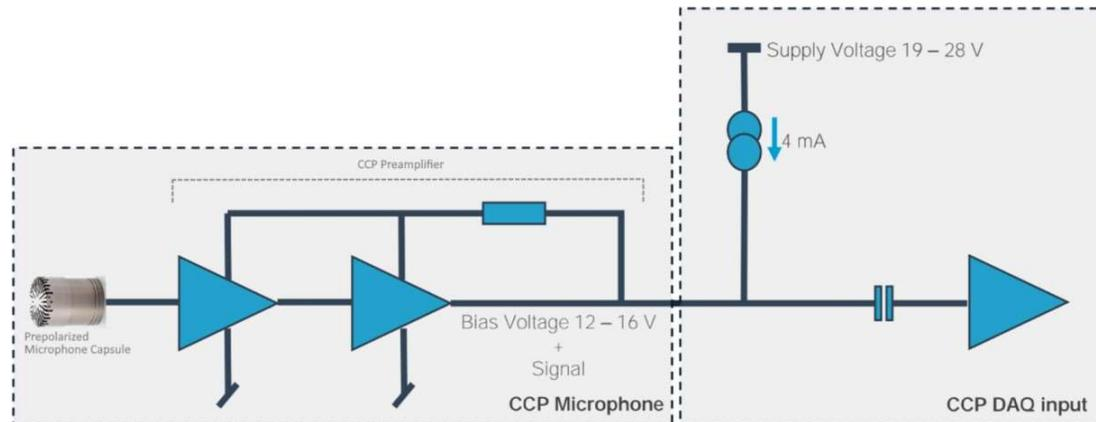
Figure 2. CCP microphone set connection layout including Prepolarized microphone capsule, preamplifier and DAQ input with built in CCP supply.
