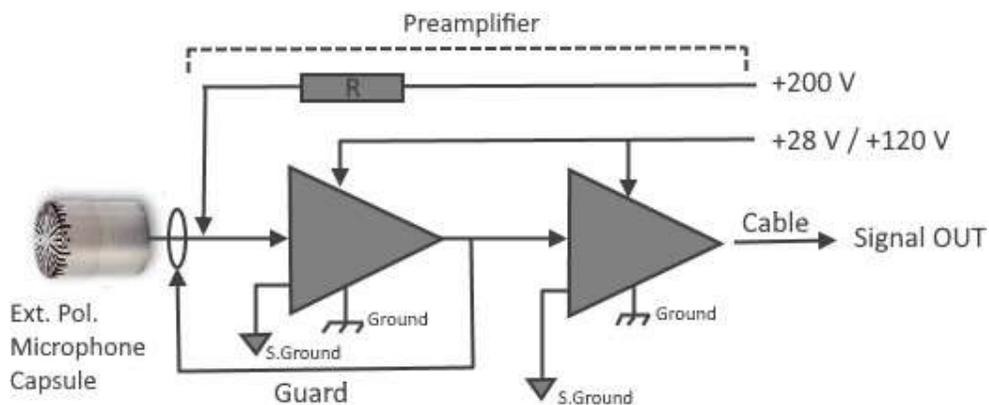
Figure 3. Traditional microphone set connection layout with Externally polarized microphone capsule.
