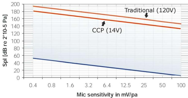
Figure 4. Comparison of upper dynamic range limits of the same microphone using a CCP vs Traditional preamplifier.
