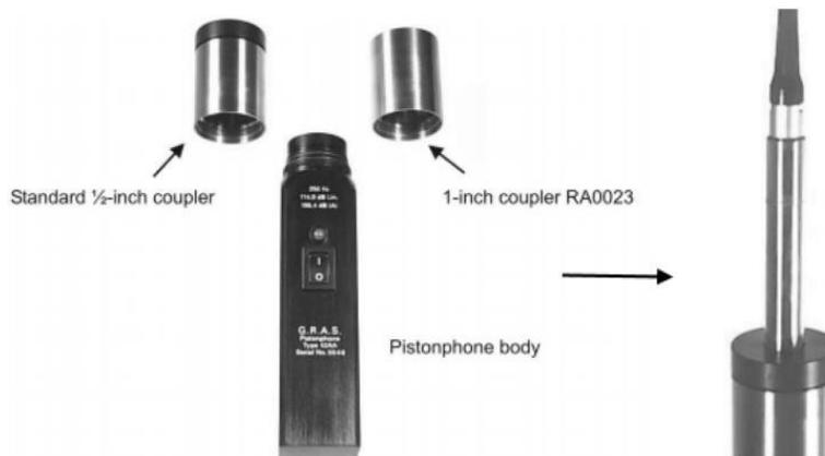
Figure 2. Left: Pistonphone with 1" and 1/2" calibration couplers. Right: 1/2" microphone set inserted in pistonphone's calibration coupler.
