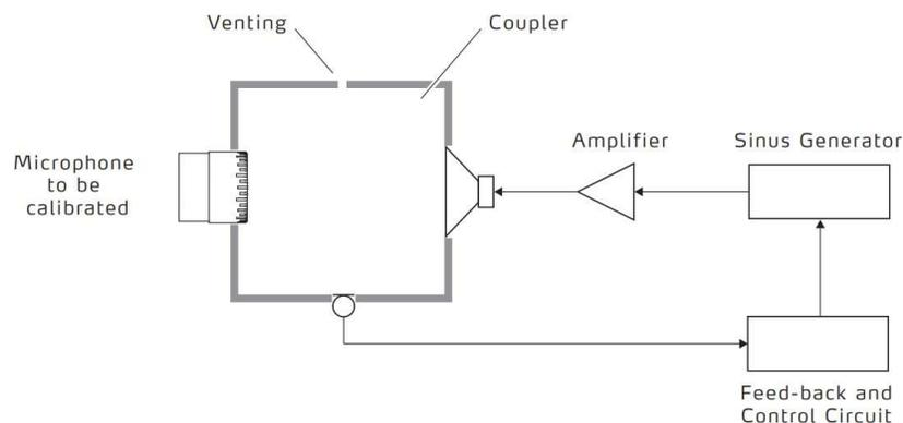
Figure 4. Simplified block diagram illustrating typical sound calibrator's principles of operation
