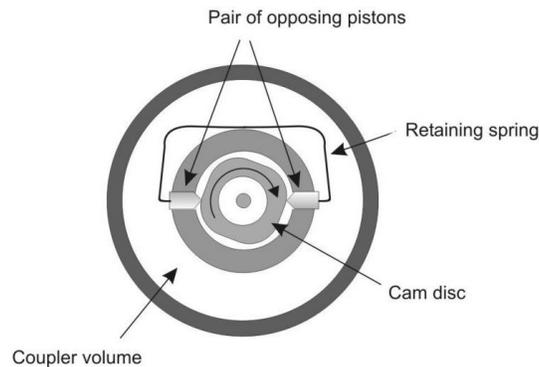
Figure 1. Principle of operation of the Pistonphone.
