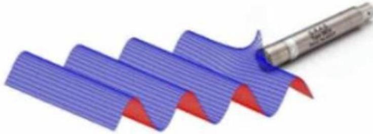
Figure 3.  $\frac{1}{2}$ " pressure microphone set exposed to high frequency sound wave with short wavelength. Diffraction effect appears.
