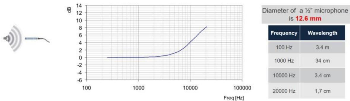
Figure 4. Pressure build-up for a  $\frac{1}{2}$ " pressure microphone pointing at 0-degree incidence from sound source in a free-field environment.
