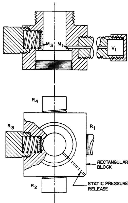
FIG. 2. Schematic drawing of Zwislocki eardrum simulator.
