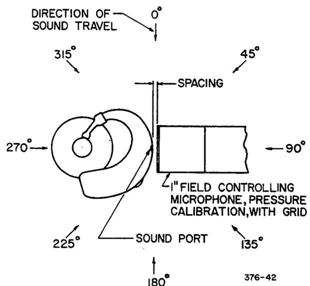
Fig. 12-1. Experimental arrangement for measuring the pressure gain of a hearing aid.
