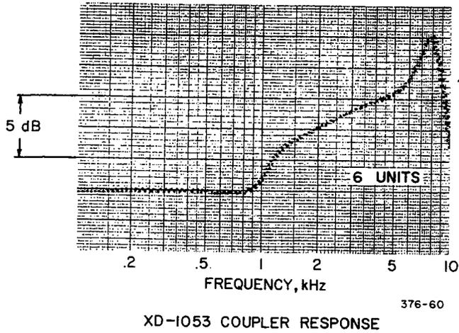
Fig. 15-11. Response of experimental ceramic earphone on XD-1053 occluded ear simulator, (6) six units.
