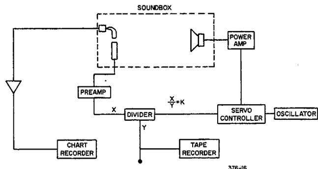
Fig. 12-5. Measurement and sound level control system for simulating the measurement of a hearing aid *in situ* without a manikin.
