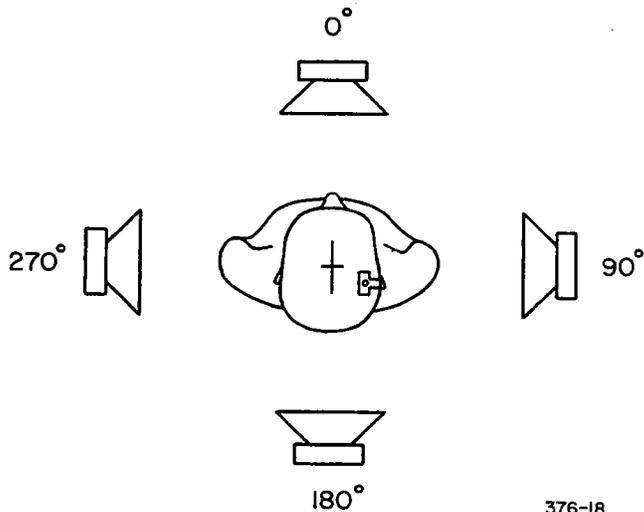
Fig. 3-3. The orientation coordinates for sound sources relative to the KEMAR manikin.
