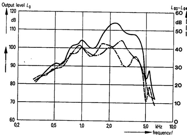
Fig. 6-4. Frequency response of a hearing aid with Type A Microphone Location. (frontal microphone through the hook). The code for the various curves is the same as in Fig. 6-3. Input level,  $L_1 = 60$  dB SPL, position of gain control to give 40 dB gain at 1 kHz under standard conditions.
