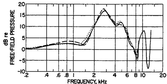
FIG. 11. Eardrum sound pressure in KEMAR showing effect of neck length on torso reflections.  $\cdots$  18.8 cm; — 17.6 cm; --- 16.3 cm.
