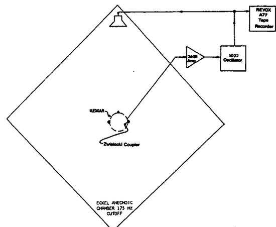
Fig. 9-7. Instrumentation to provide flat SPL at KEMAR eardrum.
