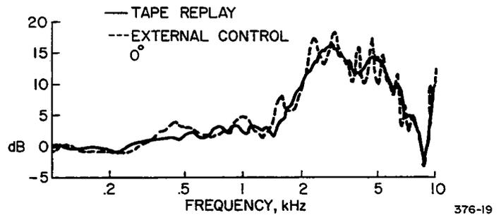
Fig. 10-5. The comparison of the open ear response of the KEMAR manikin for a tape replay free field and for control by an external microphone placed between the loudspeaker and the manikin, two feet from the loudspeaker.
