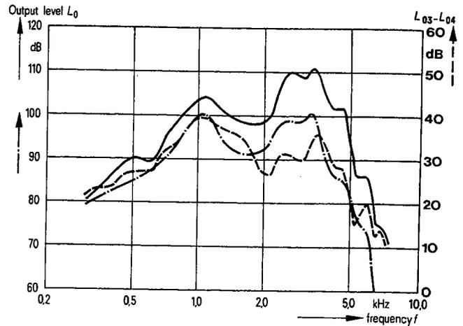
Fig. 6-5. Frequency response of a hearing aid with Type B Microphone Location. (microphone at the bottom of the case). The code for the various curves is the same as in Fig. 6-3. Input level,  $L_1 = 60$  dB SPL, position of gain control to give 40 dB gain at 1 kHz under standard conditions.
