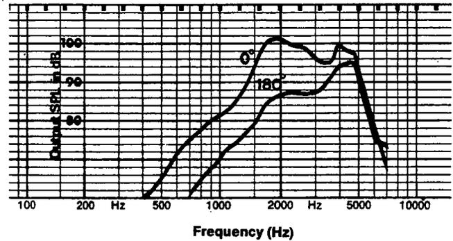
Fig. 9-10 (a). Directional ITE aid response in KEMAR using control microphone positioned 2" above center of KEMAR head.
