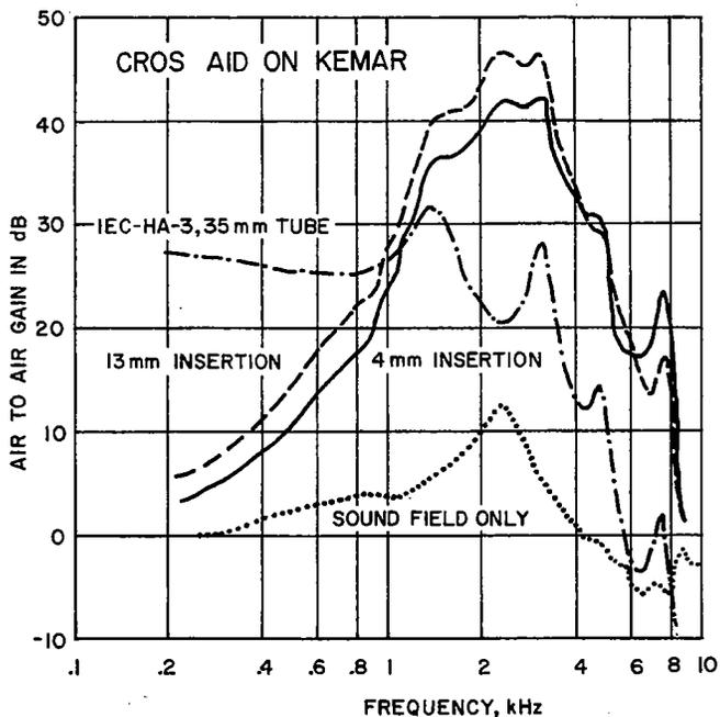
Fig. 11-3. Various gain curves for a CROS hearing aid on the KEMAR manikin and the same hearing aid measured on an HA-3, 2 cm<sup>3</sup> coupler system.
