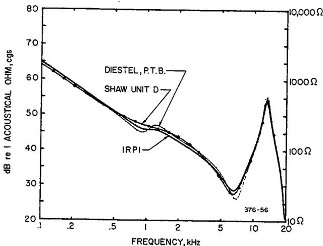
Fig. 15-12. Magnitude of input impedance for 3, two branch occluded ear simulator designs, calculated by computer model.
