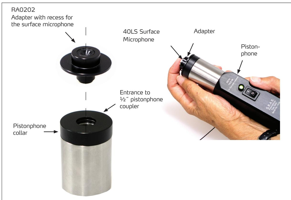
**Fig. 9.** Calibration using a pistonphone.
