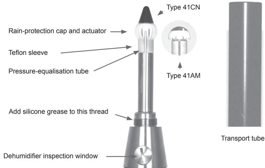
*Fig. 2.4 Showing microphone assembly - note the difference between the two rain-protection caps*
