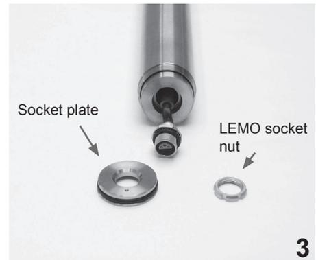
4. Remove the rubber O-ring, locking washer and nut from the LEMO socket.
