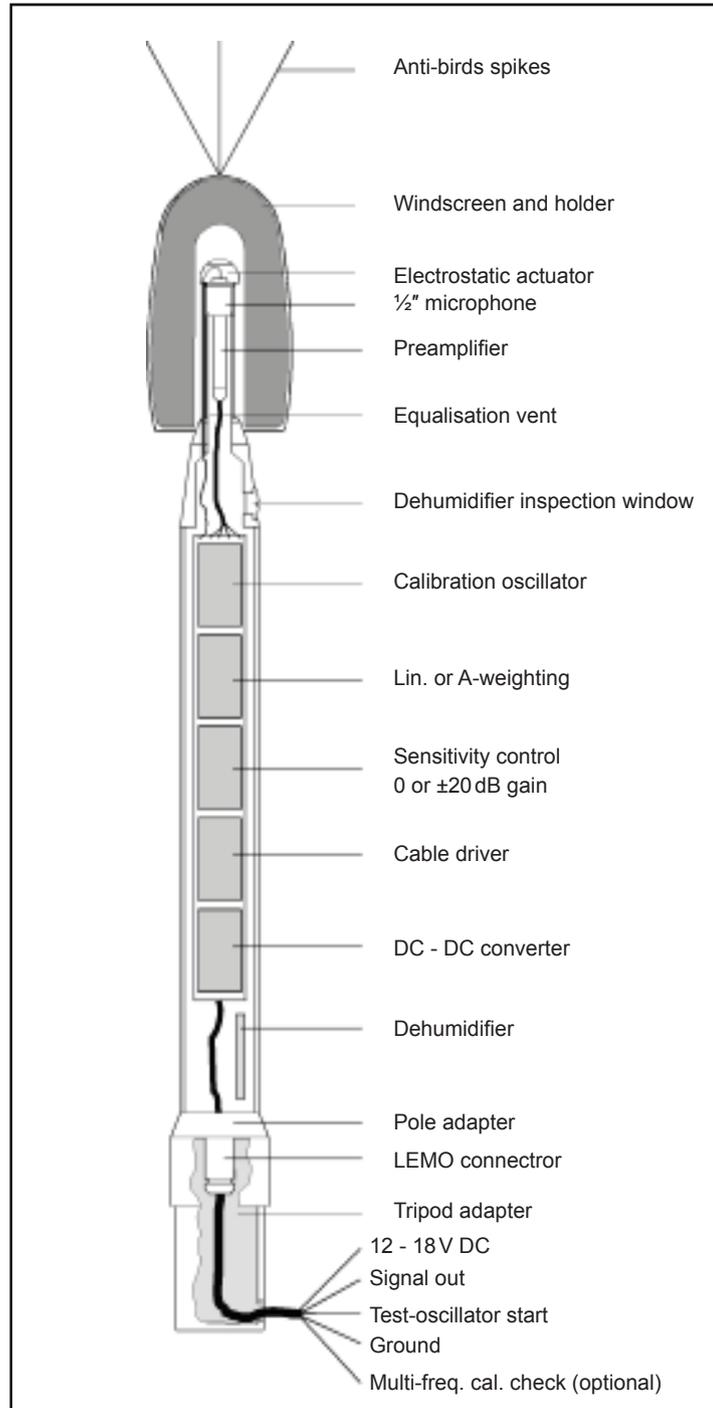
Fig. 2.1 Main components of the Outdoor Microphone System
