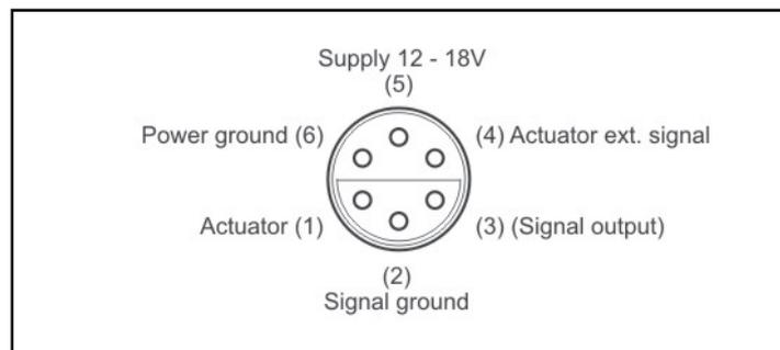
Fig. 5.2 LEMO socket output connections (external view)
