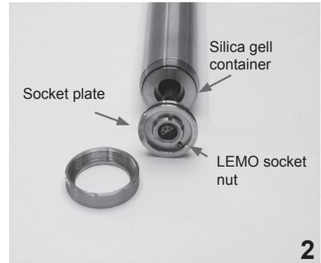
3. Unscrew the LEMO socket nut and remove the socket plate ⑤.
