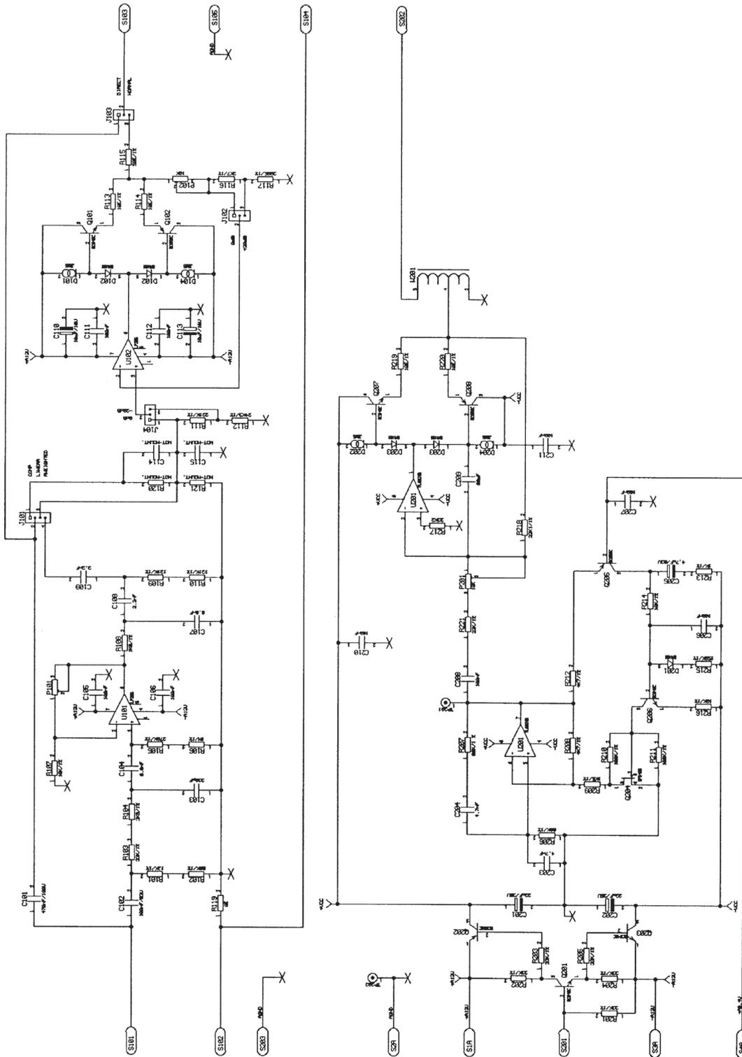
Fig. 8.1 Circuit diagram for signal conditioning
