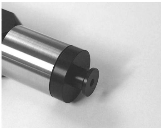
Fig. 3.5  $\frac{1}{8}$ " microphone adapter inserted in the coupler
