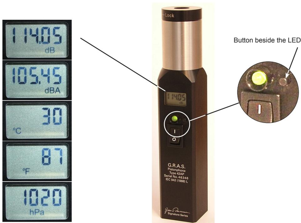
Fig. 1.1 Pistonphone Type 42AP shown with display examples
