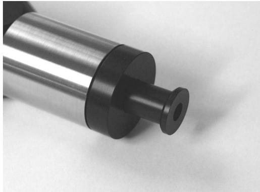
Fig. 3.4 ¼" microphone adapter inserted in the coupler
