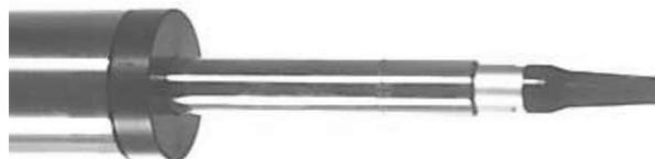
Fig. 3.3 ½" microphone inserted in the coupler
