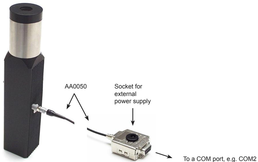
Fig. 4.1 Pistonphone connection to computer
