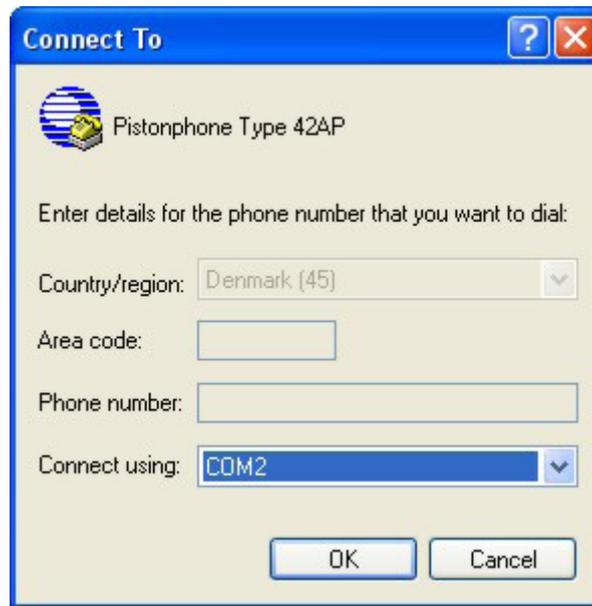
Fig. 4.2 Selecting the COM port in use, e.g. COM2
