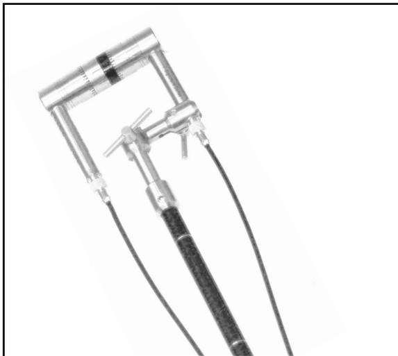
*Fig. 3.2 Symmetrical setup using the 12-mm spacer*
