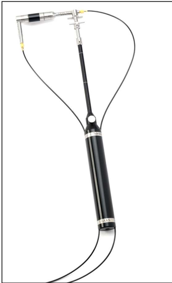
Fig. 1.1 The CCP Intensity Probe Type 50GI
