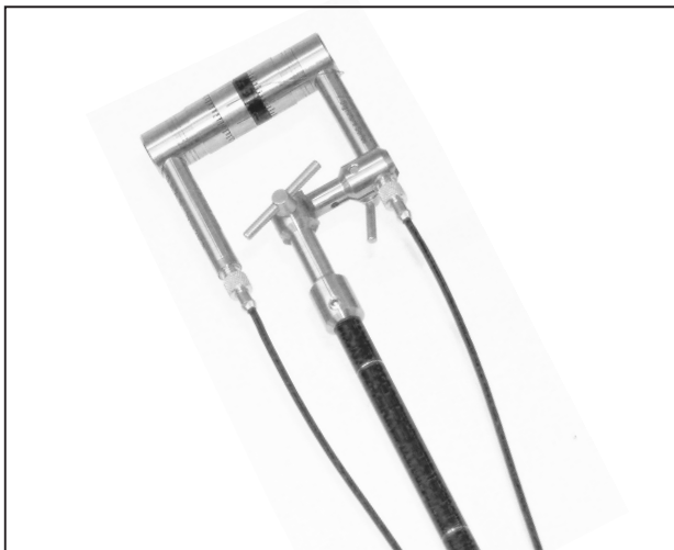
Fig. 3.2 Symmetrical setup using the 12-mm spacer
