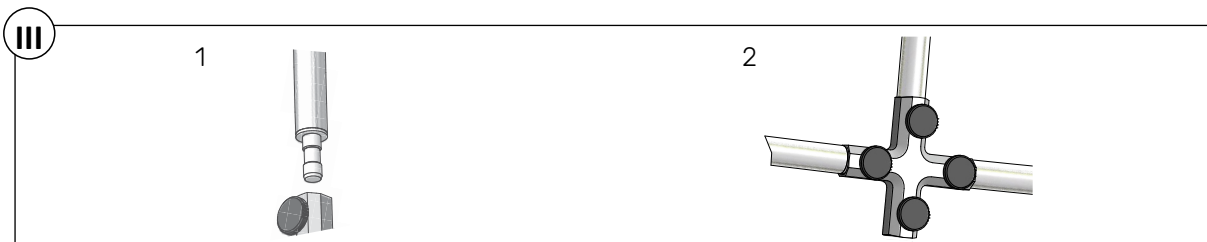
Fig. 24. Attaching vertical poles to the B-layer circle.
