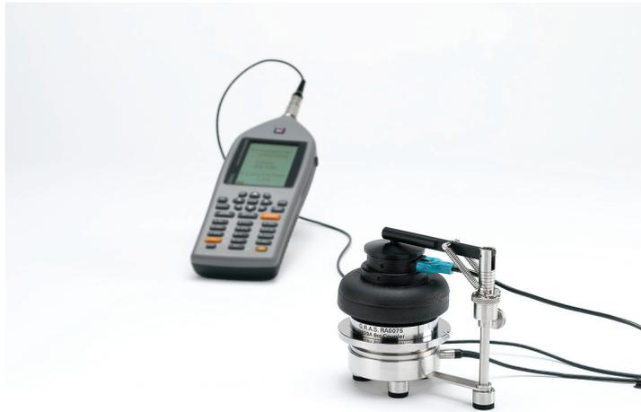
*Fig. 3. A typical setup with supra-aural earphones.*
