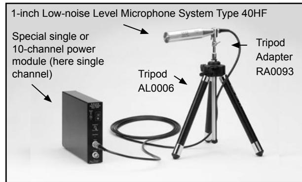
Fig. 2 A complete single-channel low-noise level measuring system
