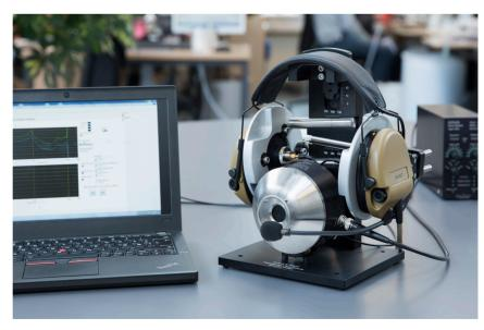
The GRAS 45CC-7 with ear simulator and %" prepolarized measurement microphone and the T5 Invisio Headset.
