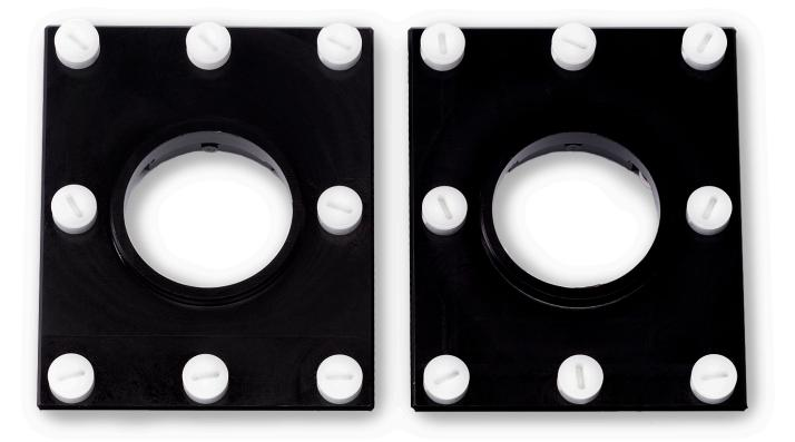
Kit with plastic ear holder plates and plastic ear canal extensions. For test of binaural hearing aids which are based on radio frequencies.
