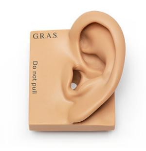
Anatomically shaped concha and ear canal Improved fit and repeatability Outer pinna with improved collapsibility Resilient mounting KB5001 is a left anthropometric pinna for KEMAR for accurate and repeatable testing of headphones and earphones. It has anatomically correct ear-entrance and ear-canal with correct soft ear helix and provides perfect sealing and insertion accuracy forheadphones and earphones. The hardness is 35 Shore 00
