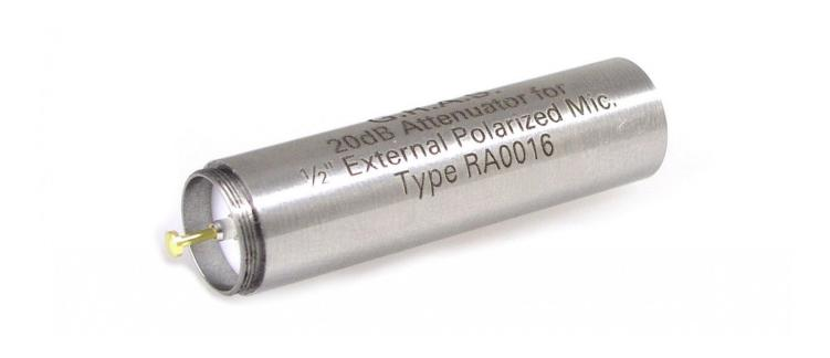
Length: 47.5 mm Diam.: 12.70 mm **Recommendation:** Choose a microphone with low sensitivity instead of using the RA0016. The RA0016 is a 20 dB attenuator for inserting between a 1/2" microphone and preamplifier. It will attenuate the output signal of the microphone by 20 dB in order to avoid overloading the preamplifier. The RA0016 is useful when measuring very high sound pressure levels using a preamplifier with limited dynamic range.
