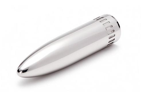
Length: 54.0 mm Outer diameter: 13.2 mm Threading (mic. protection grid threading): 12.70-60 UNS-2 Material: Stainless steel Weight: 45 g The RA0020 is specially designed and optimized for use with 1/2" microphones for sound pressure measurements, when high speed wind comes from one known direction e.g. in a wind tunnel.
