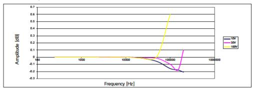
The Frequency response for the O VDC and 200 VDC outputs, 1 meter RG58 cable, 10, 30 and 100 V RMS.
