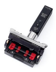
Standard: IEC 61043 Special feature: Calibration coupler with two matched calibration chambers for GRAS Rugged Intensity Probes. The 51AC Sound Intensity Calibration Kit is a ready to use kit for sensitivity and phase calibration of GRAS Rugged Intensity Probes (50AI-LP, 50GI-P, 50GI-RP). The kit consists of a calibration adapter with two calibration chambers, a GRAS 42AA Pistonphone, Class 1, and a GRAS ZC0002K Barometer.
