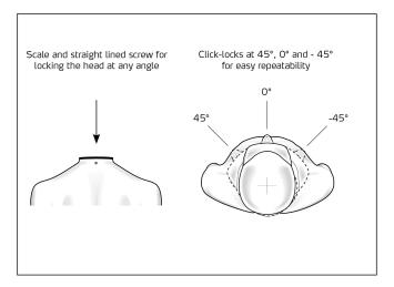
A scale around KEMAR's neck indicates the head angle and allows for repeatable measurements.
