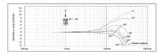
Free-field corrections for various degrees of incidence
