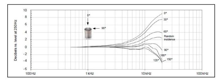
Free-field corrections for different angles of incidence
