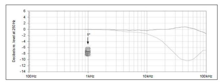
Typical frequency response (without protection grid). Upper curve shows free-feld response for 0°, lower curve shows pressure response.
