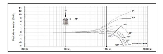
Free-field corrections for various degrees of incidence
