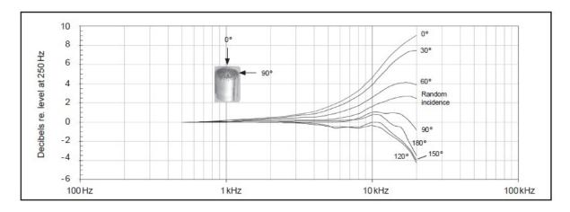
Free-field corrections for different angles of incidence
