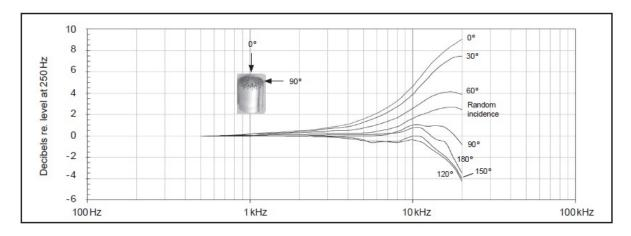
Free-field corrections for different angles of incidence
