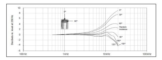
Free-field corrections for different angles of incidence
