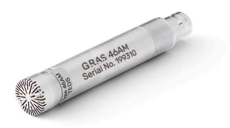
Freq range: 3.15 Hz to 31.5 kHz Dyn range: 25 dB(A) to 149 dB Sensitivity: 14.5 mV/Pa Use: For general acoustic diagnostics The GRAS 46AM is a 1/2" Constant Current Power (CCP) free-field microphone set for measuring medium sound pressure levels at a wide range of frequencies. It is terminated with a BNC connector and is TEDS compatible. The equivalent traditional 200 V LEMO type is <u>GRAS 46AC</u>.
