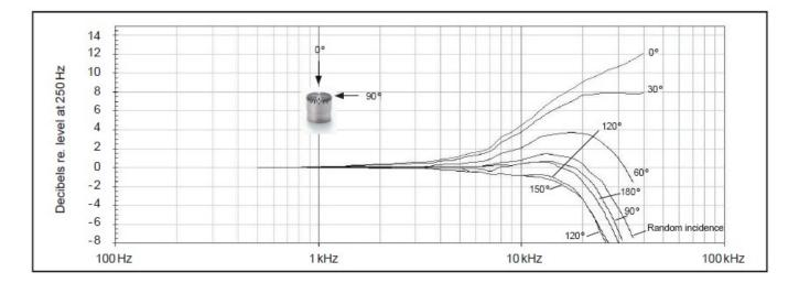
Free-field corrections for different angles of incidence
