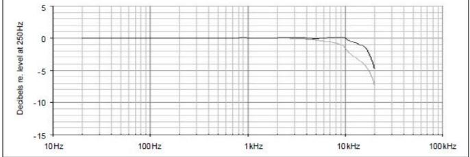
Typical frequency response. Upper curve shows response in a diffuse sound field (random incidence), lower curve shows pressure response.
