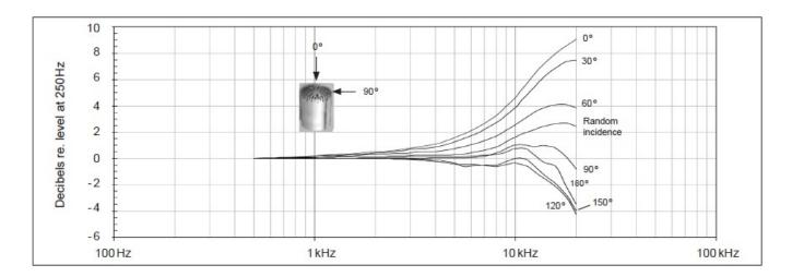
Free-field corrections for different angles of incidence
